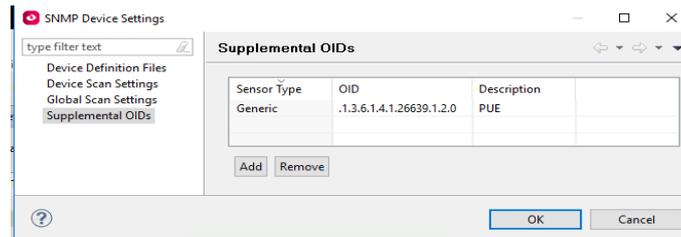
Under Monitoring (Device or Map view) right click on DCO Server and select “Request Device Scan”. Wait a few seconds then “View Device Sensors” – you should now see PUE
